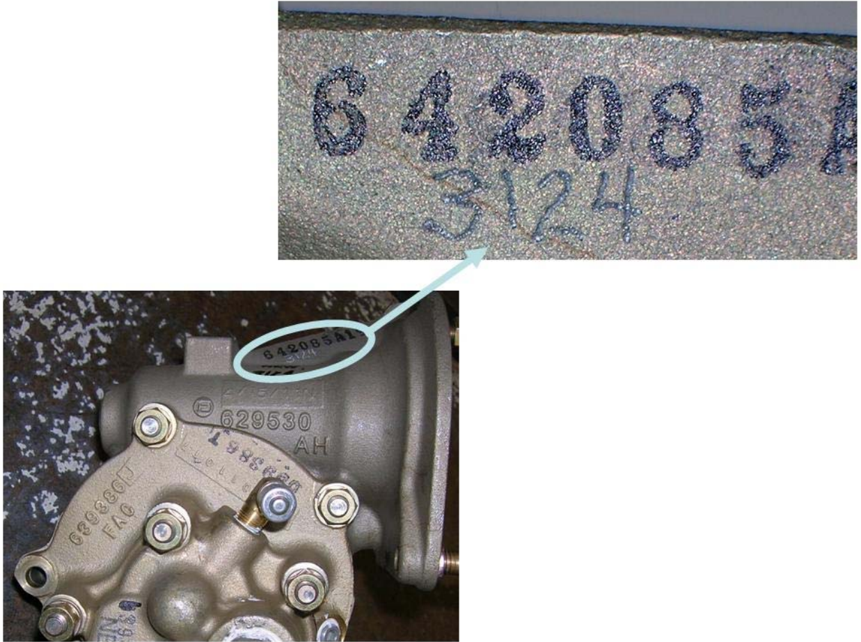
FIGURE 1 – Example of vibro-peened manufacturer code
